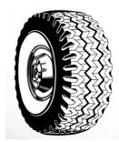
Tire Care – If a vehicle is left stationary for too long, the tires could develop flat spots from weight of the vehicle pressing down on the tires' treads. This occurs at a faster rate in colder temperatures, especially with high -performance or low-profile tires and in severe cases, a flat spot
