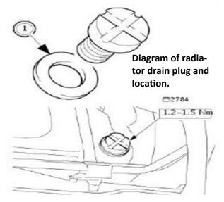
plug in till the final fill and tore up the old one pretty bad with the repeated drains and fills. The drain plug is only supposed to be tightened to 9 in-lbs., so don't over tighten it.
