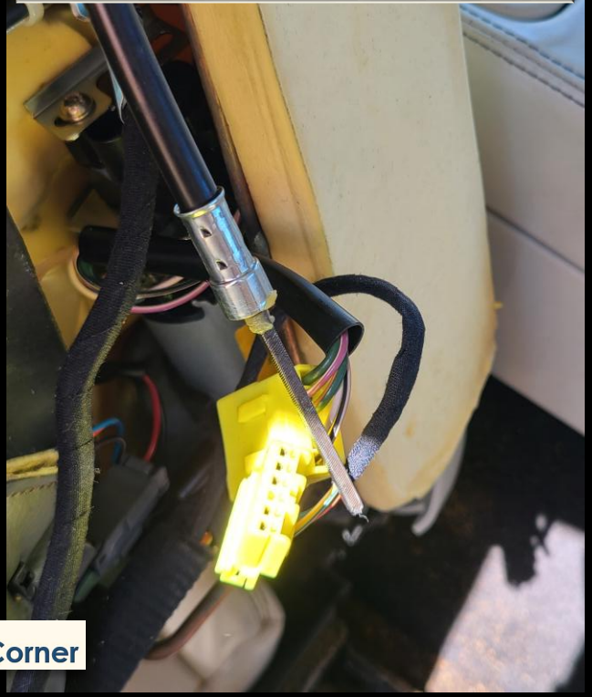
End of headrest motor cable with crimp fitting pulled out for access
