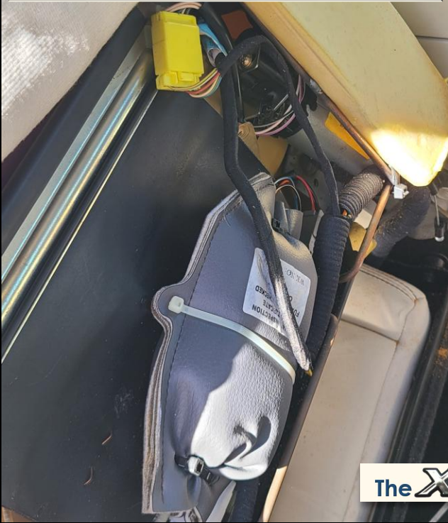
Driver's seat with leather detached at bottom and pulled up—headrest motor is just below and to the right of yellow connector
