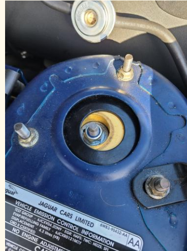
Shock bolt off-center in URO aftermarket mount
