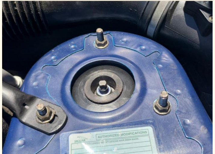
Correctly-installed upgraded shock mounts
