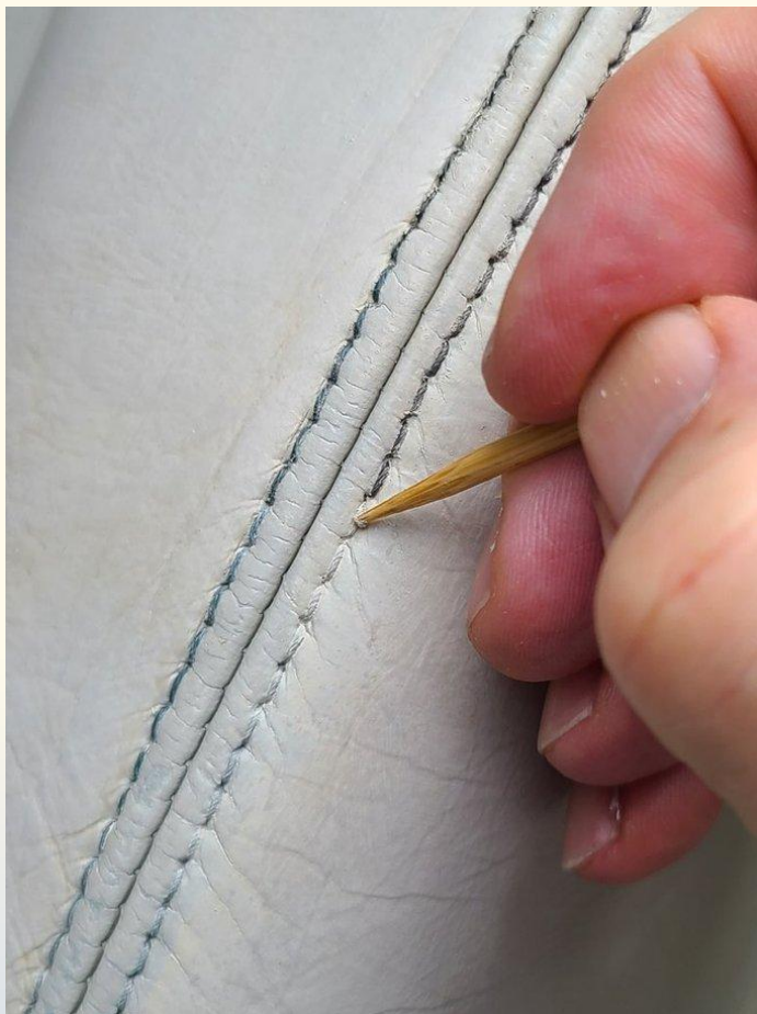
Using a wooden skewer to scrape off uncured dye from contrasting stitching
